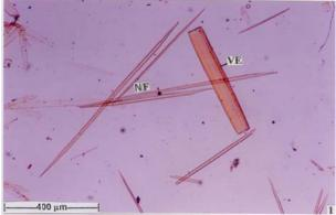
Fig. 6.1 Narrow Fibre and one narrow vessel element
