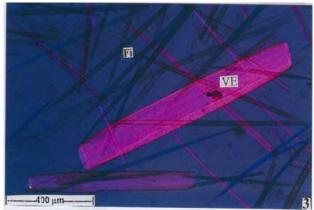
Fig. 5.3 Vessel Element and fibres under polarized light microscope
