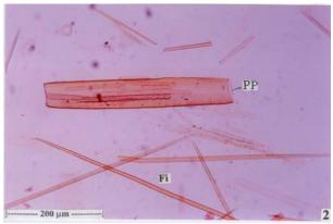
Fig. 6.2 One wide vessel element and narrow fibres
