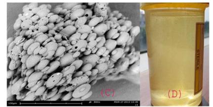
Figure 3. SEM photography C showing the microsphere shape and photography D showing the appearance of microspheres enriched syrup
