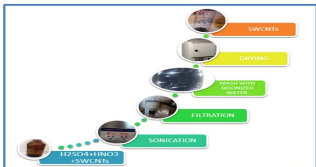
Figure 1: Steps of carbon nanotubes purification and carboxylation
