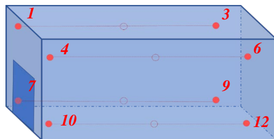
Figure 5. The diagram of EDLMs arrangement during temperature mapping: a) before quantity reduction of EDLMs; b) after quantity reduction of EDLMs
