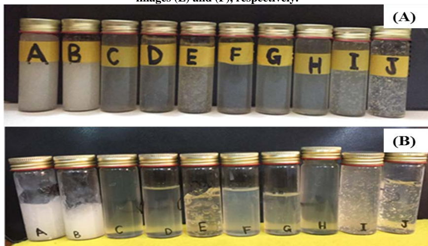
Figure 3: Visual appearance of drug loaded hydrogel in different concentration of four types of gelling agents Xanthan Gum (A & B), Carboxymethylcellulose (C, D, E), HPMC (F, G, H), Carbopol 974P (I, J) to prepare dermal delivered hydrogel dosage form. (A) Freshly prepared formulations. (B) After three months.
