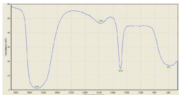
Figure (1): Fourier Transform Infra-Red Spectroscopy (FT-IR) analysis of ZrO_2 nanoparticles.
