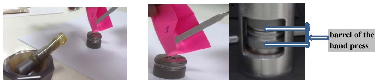
Figure (2): Placement of mixture in the die
