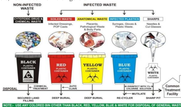
Fig 5 Collection of BMW in different coloured bags for easy handling and disposal (Sources: Times Delhi Magazine, 2017/05/16/staffers ignorance ruins waste management)
