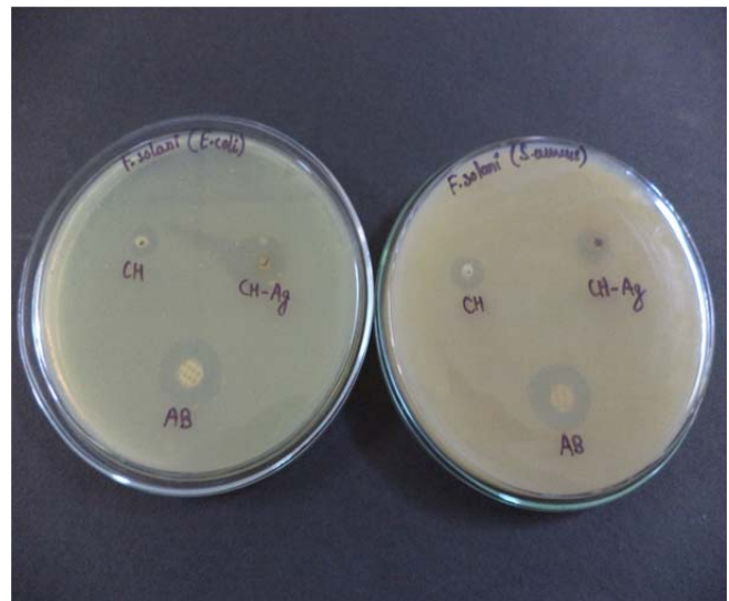
Fig.16 Comparative study of the antimicrobial activity of the polysaccharides (Chitin) and its bionanocomposites
