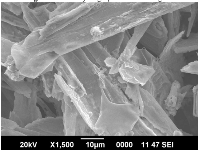
Fig.14 SEM Image showing the needle shaped surface of Chitosan AgNP
