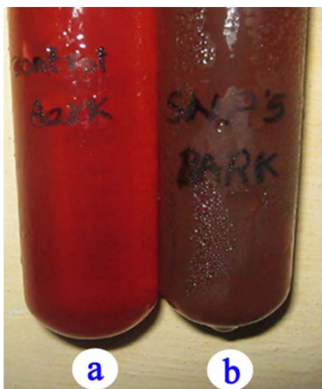
Fig. 1 Synthesis of SNPs from stem bark of A. digitata colour change pattern a. Plant extract b. Synthesized SNPs
