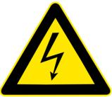
This sign, 'high voltage' means voltage at such a high level that if any living organism comes in contact with the electricity, the electricity will cause harm or even death.
