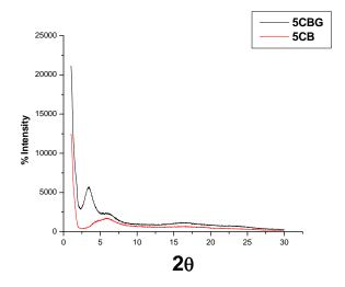
Figure 2. XRD spectra of 5CB & 5CBG.
