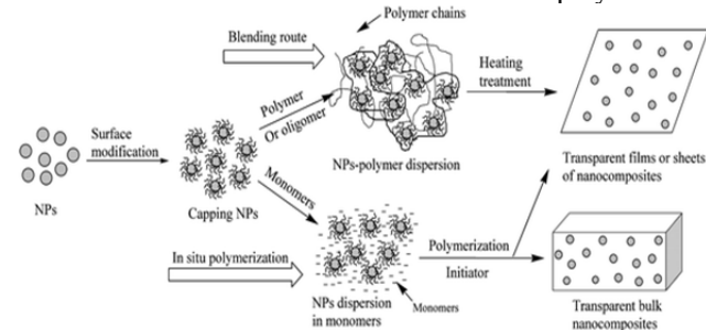
Fig 2- Preparation of Polymer nano composites using nanoparticles
