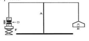
fig.2.bloadhesive force measuring device, (A)modified balance,(B)weights,(C)glass vial, (D)gellan based gel,(E)chicken cheek mucous membrane,(F)height adjustable pan.
