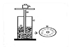
Figure 1.diagramatic representation of apparatus used for finding gel strength.
