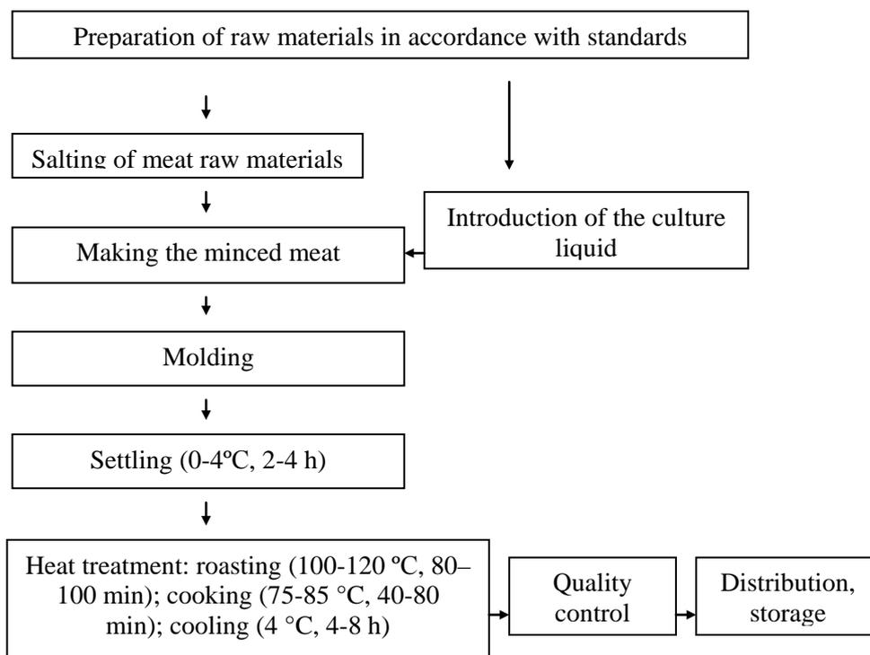
Figure 1 — Technological Scheme for the Production of Cooked Sausages
