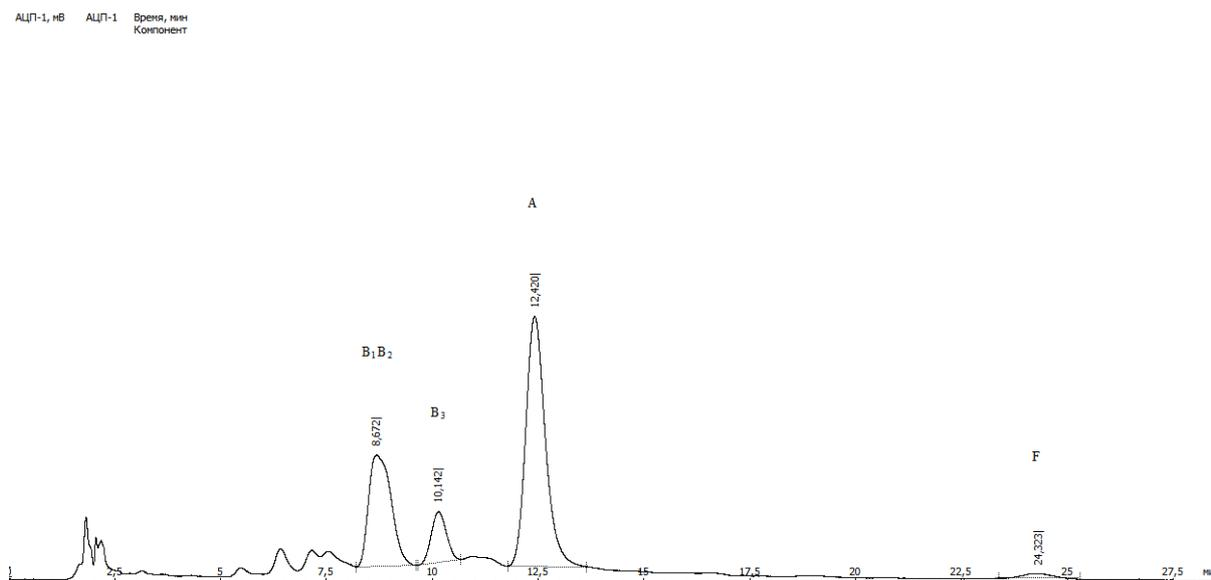
**Figure 3.** Chromatogram with EDTA added to the tested solution of 0.5% concentration.
