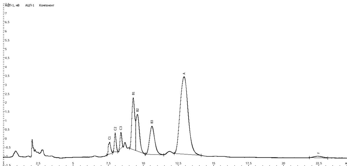
Figure 1. Separation of zinc bacitracin components with the help of HPLC.
