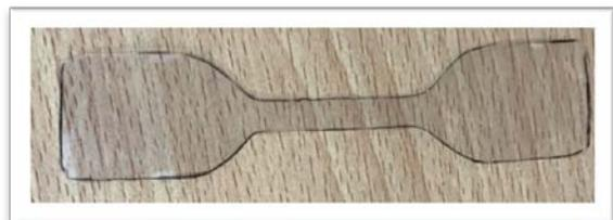
**Fig (1) Sample Cut into Dumbbell Shape for Mechanical Properties.**
