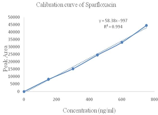
Fig. 4: Calibration curve for Sparfloxacin
