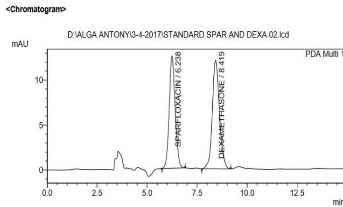
Fig 3. Typical chromatogram obtained for the Sparfloxacin and Dexamethasone
