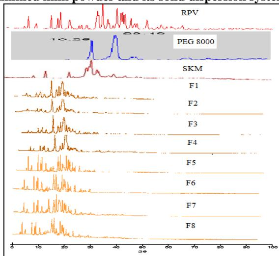
Figure 7: XRD spectra of rilpivirine, PEG 8000, skimmed milk powder and solid dispersion systems.
