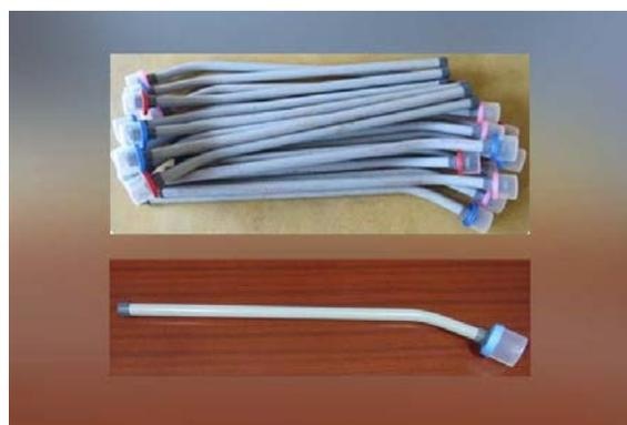
Fig. 14: Stack probe for detection of spoilage in turmeric
