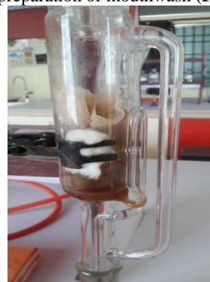
Figure 1: Soxhlet extraction of the herbal components.
