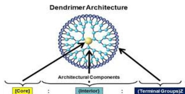
Figure2. Architecture of a dendrimer.
