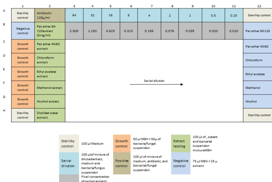
**Figure 1: Design of the 96-well plate for colorimetric broth microdilution antimicrobial assay of crude extracts**
