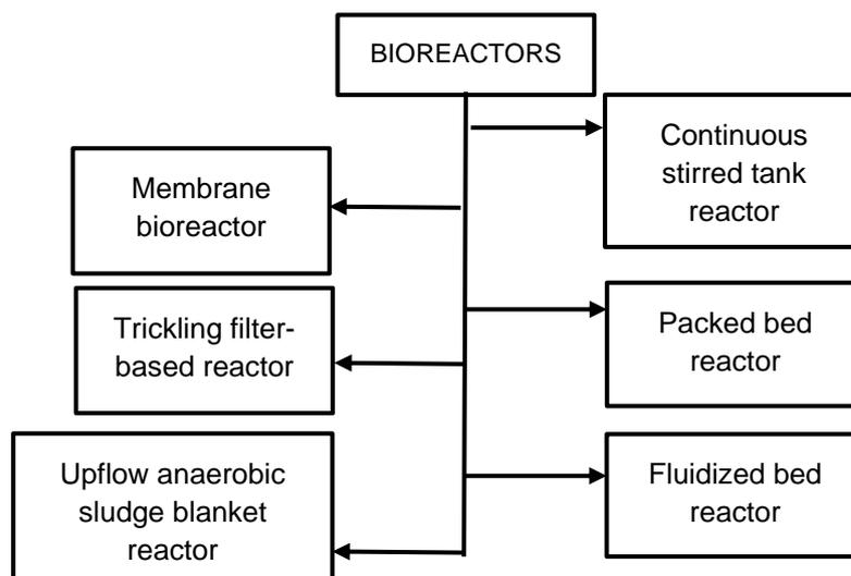
Fig 3. Various bioreactors used for biohydrogen production
