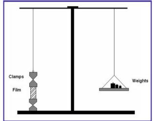
Modified tensile strength tester.
