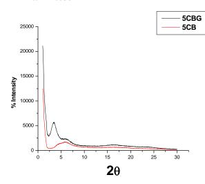
Figure 2. XRD spectra of 5CB & 5CBG.
