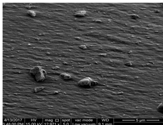
Fig. 3: SEM micrograph of biogenic silver nanoparticles. The shape of AgNPs was spherical and homogenous, size between (64-100nm).
