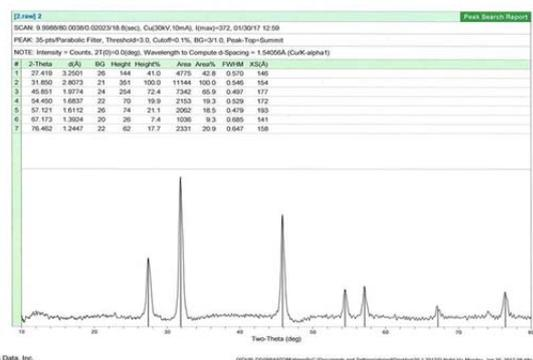
Fig.2 : XRD analysis of Biosynthesized nanoparticles using *P.agglomerans* (average diameter 16.73nm)
