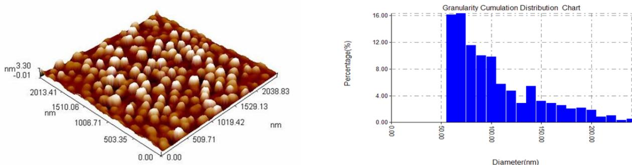
Fig.5. Atomic Force Microscopic analysis of biosynthesized silver nanoparticle from *P.agglomerans* (Average Diameter: 98.78 nm)
