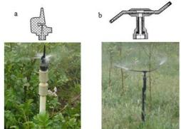
Figure 3 – Sprinkling nozzles designed by KazSRIWE LLP (a – spray nozzle; b – carousel nozzle)
